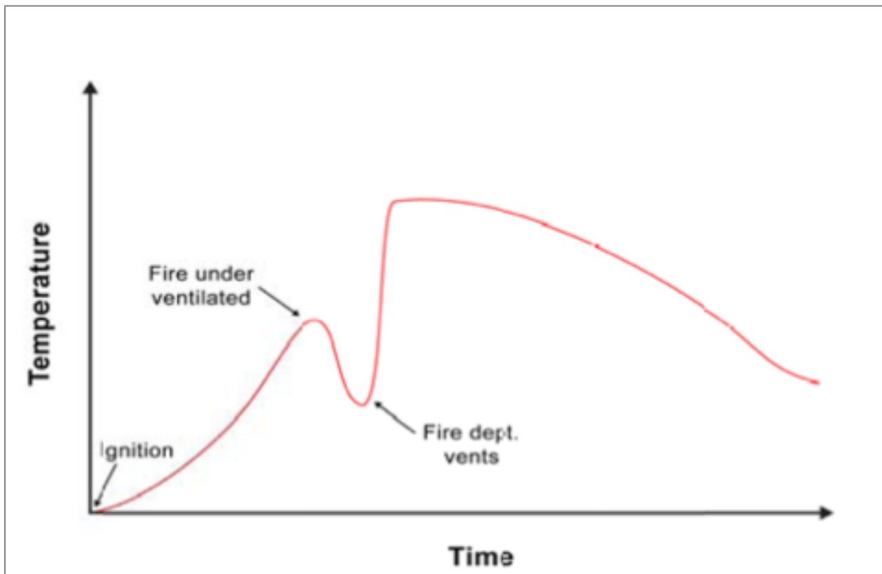
Figure 29: Ventilation Controlled Time Temperature Curve
